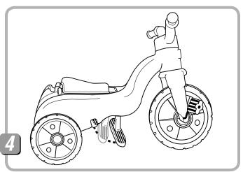
• Rotate the footrest up toward the rear wheels and snap it into the recess in the underside of the frame.
